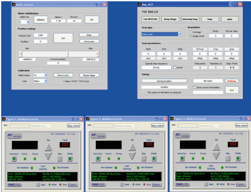
Fig. 4.11 Graphical user interfaces (GUIs) of the software components written for controlling the experimental setup. All programs were written in MATLAB. 'sm32_control' is the GUI for controlling the delay stage. 'MGMotorControl' is the software for driving the wave plate rotation stage and was provided by the manufacturer. It is loaded into MATLAB for each utilised rotation stage (from left to right: HWP1, HWP2, QWP). On the upper right hand side, the GUI 'daq_tof2' is displayed that is used for linking the previous GUIs. It is described in more detail in the text
