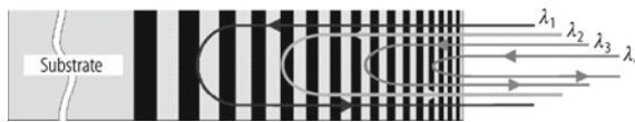
Fig. 3.3 Chirped mirrors are dielectric multilayer mirrors. Due to a modulation of the period of the multilayer stacks, longer wavelengths travel further into the mirror before being reflected. This is due to the constructive interference condition for the partial waves of one spectral component reflected at the interfaces between low and high refractive index layers [6]. As a result, longer wavelengths travel a longer optical path upon reflection than shorter ones and hence a negative dispersion is induced. (Reprinted from [9], with permission from Springer Science+Business Media)
